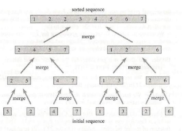
**Figure** The operation of merge sort on the array A = (5, 2, 4, 7, 1, 3, 2, 6). The lengths of the sorted sequences being merged increase as the algorithm progresses from bottom to top.
